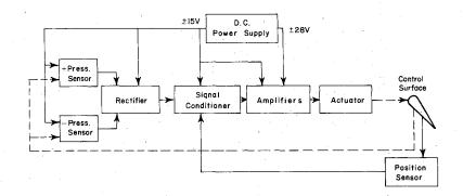
Fig. 2 System flow diagram.
