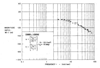
Fig. 4 Position and  $\Delta P$  command bode plots for  $|\delta_F|=15$  deg and dynamic pressure = 20.1 psf.
